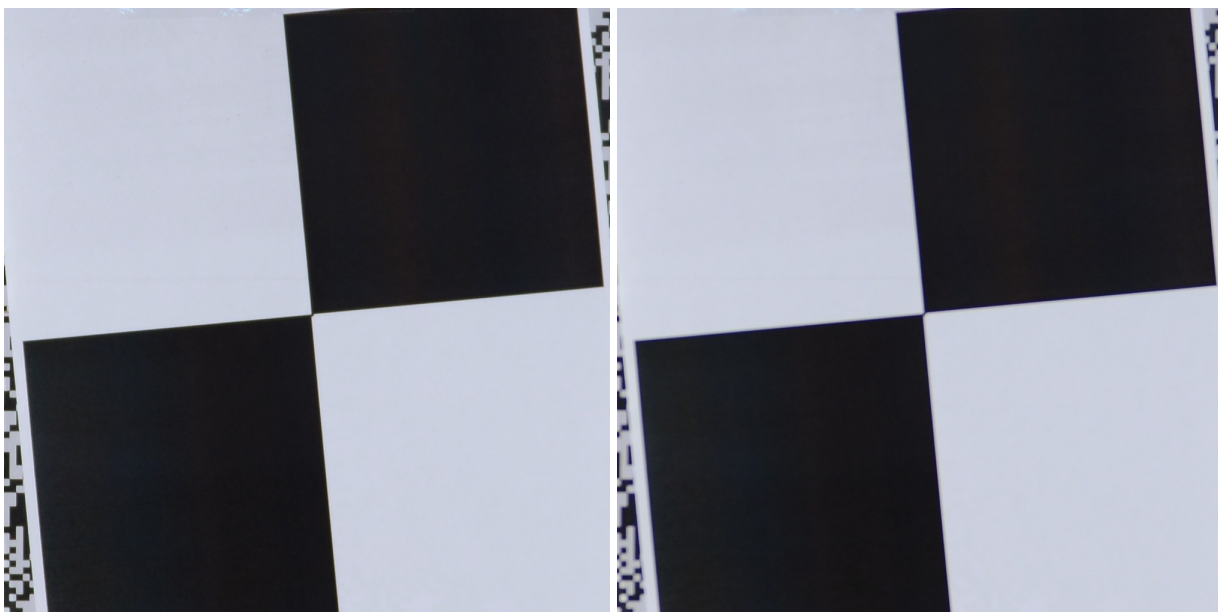
Fig. 14 Test shot at AFMA=-20 (left, top) and AFMA=+20 (right, bottom).
